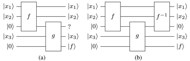
Fig. 1. An example of mapping two parts into quantum circuit; (a) does not uncompute the first part, leading to an unknown *garbage* state, (b) does uncompute the first part by computing it again in reverse order.
